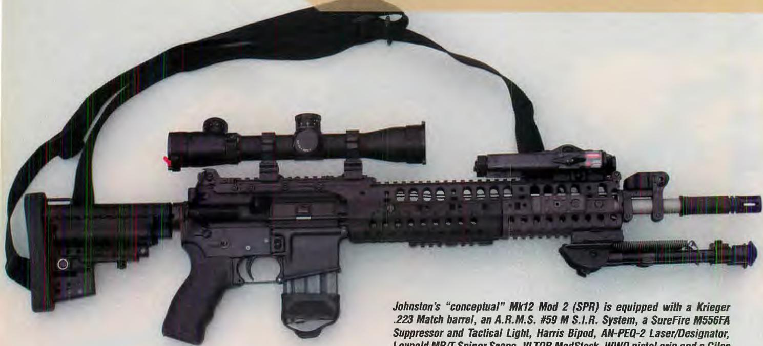
Johnston's "conceptual" Mk12 Mod 2 (SPR) is equipped with a Krieger .223 Match barrel, an A.R.M.S. #59 M S.I.R. System, a SureFire M556FA Suppressor and Tactical Light, Harris Bipod, AN-PEQ-2 Laser/Designator, Leupold MR/T Sniper Scope, VLTOR ModStock, WWO pistol grip and a Giles Tactical Sling.
