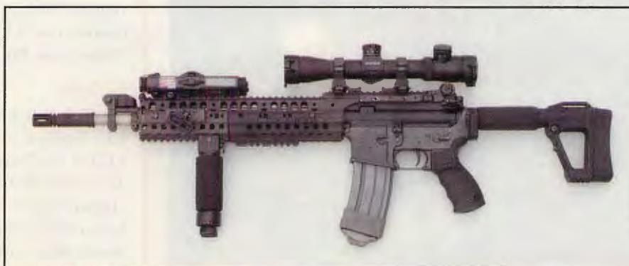
Here Johnston's rifle is seen with the ACE SOCOM 16 retractable stock, ERGO pistol grip and the GripPod vertical foregrip/bipod. Fully equipped, the "Mk 12 Mod 2" weighs in at about 9.5 pounds.
