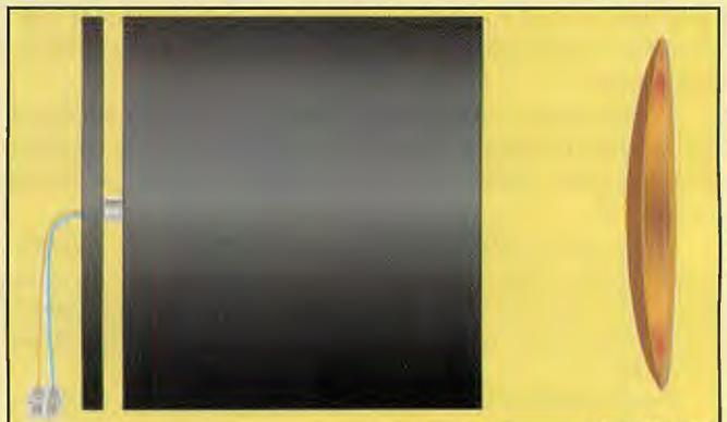
welded steel plate drilled in the centre to take a blasting cap.
